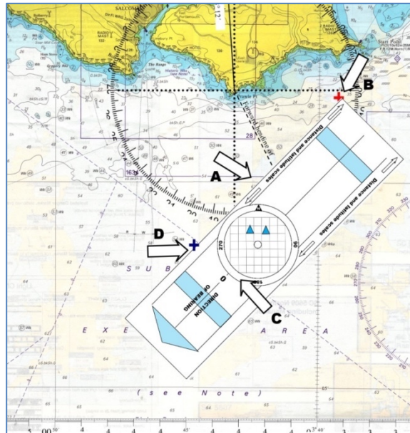
Figure 7-12 Plotting the bearing and distance between two points
