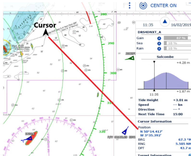
Figure 7-11 Cursor information on the radar
