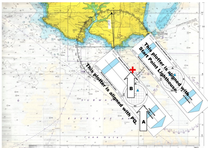
Figure 7-10 Plotting a bearing and distance on the chart
